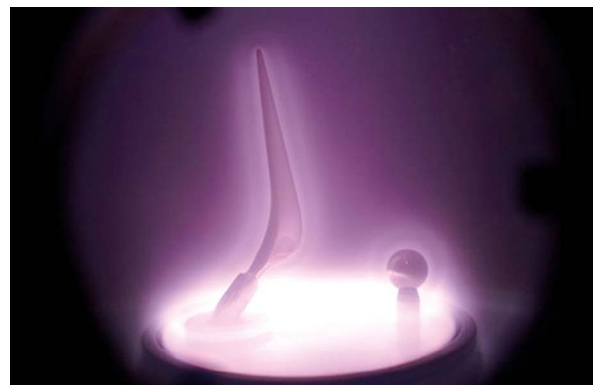
Figure 3. The prosthesis during surface modification with the Si-DLC layer using the PA RF CVD method
