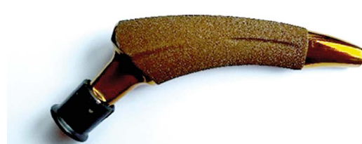
Figure 2. Macro photo of the Ti6Al4V alloy prosthesis after the modification process with porous titanium using the APS method and the Si-DLC coating using the RF-PACVD method
