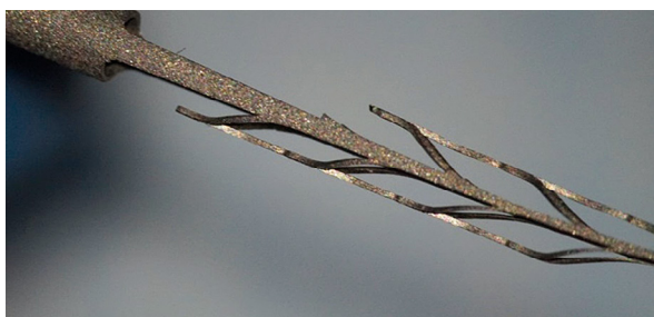
Figure 3. Example of SAF file damage: separation. Magnification: 2.5. OPMI Pico, Zeiss
