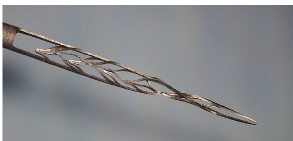
Figure 4. Example of other SAF file deformation: twisting of file tip. Magnification: 2.5. OPMI Pico, Zeiss
