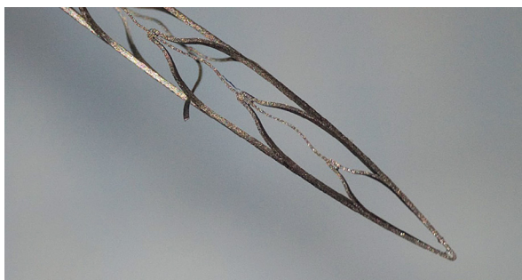
Figure 2. Example of SAF file crack. Magnification: 2.5. OPMI Pico, Zeiss
