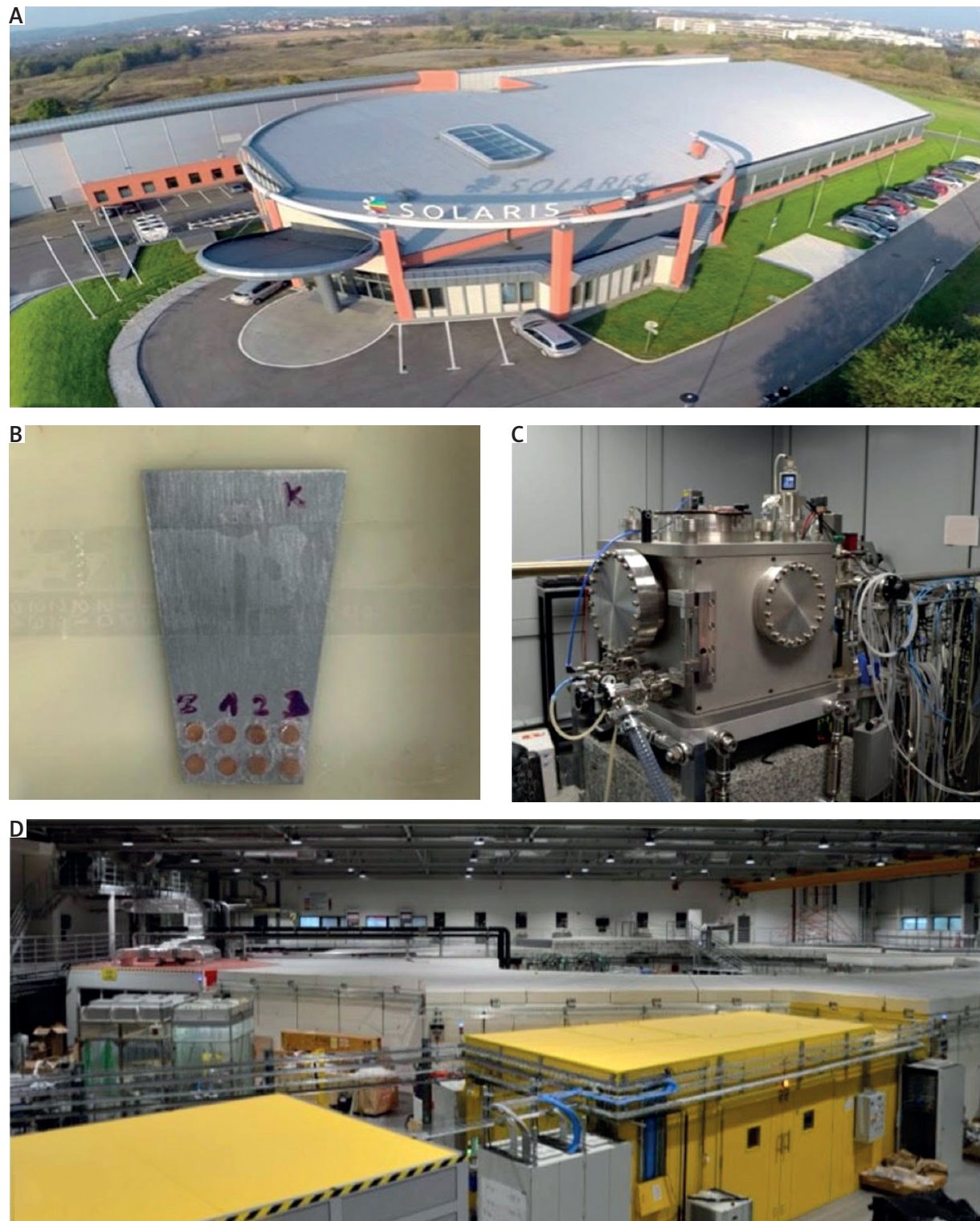
Figure 2. A – Aerial view of the “SOLARIS” Centre. B – Samples mounted for scanning transmission microscopy. C – Scanning transmission X-ray microscope at a synchrotron beamline. D – Research hall at the SOLARIS synchrotron with various beamline stations
